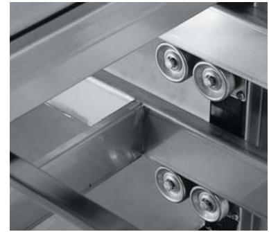
Oversized stainless steel drawer guides with heavy duty double skate rollers and stainless steel bearings can withstand 275 lbs. (125).
