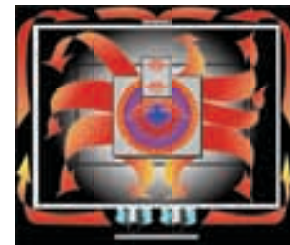
Imperial's Turbo-Flow System provides even cooking throughout the entire oven - less shrinkage results in juicier, better tasting products
